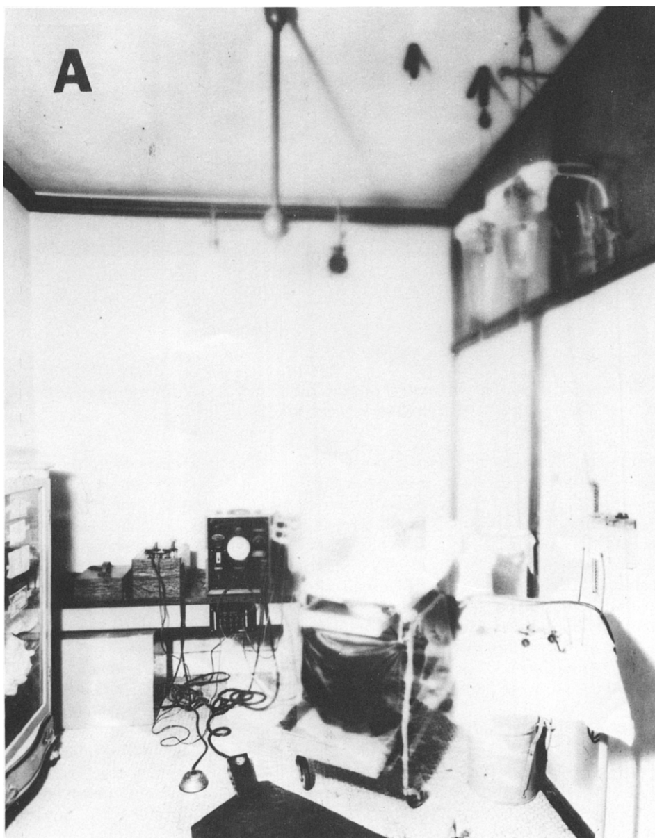
FIGURE 3. (A) Office resection operating room in Greenville (about 1928): A resection endotherm for cutting was first generator obtained for resection, other generator is teletherm diathermy generator used for coagulation of bleeding. Note double-throw switch used to change from one current to other manually. (Triple pole electromagnetic switch is direct descendant of this switch.) (B) Davis examining room in Greenville about 1930.
